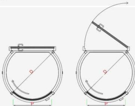
The Vigrel Combi is a compact, high-security portal that combines a curved sliding door on one side with an existing fire-rated swing door on the other. This smart retrofit solution transforms a standard doorway into a fully controlled mantrap, ensuring maximum protection while maintaining fire compliance.
